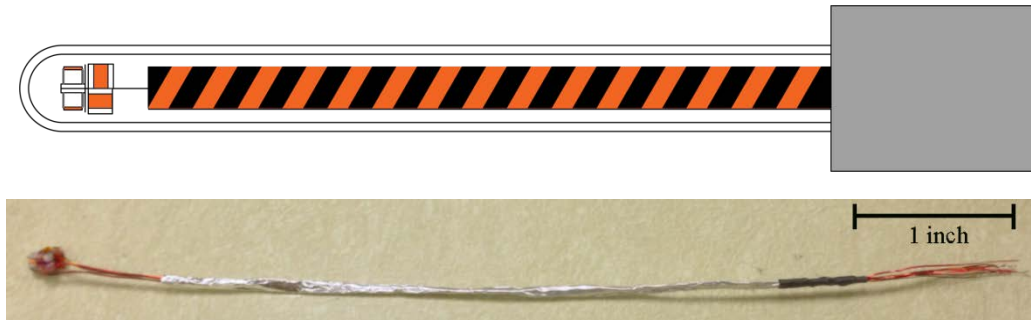
Figure 4: (top) schematic of copper tape wrapping around the plastic retention. (bottom) aluminum foil sheilding separating each wire
